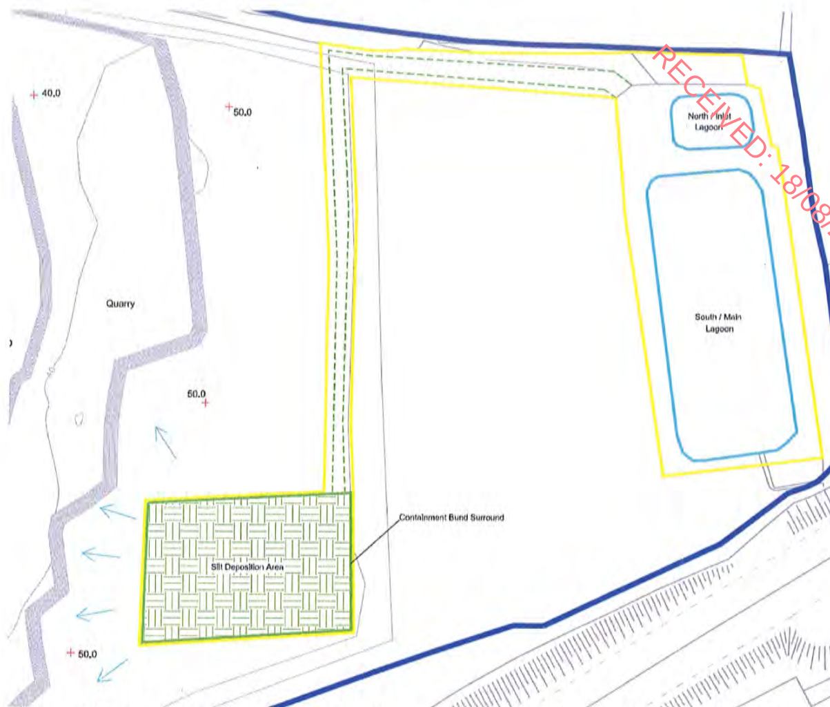
Fig 1. - Sketch showing excavation, haul routs and deposition area for cleaning process.
